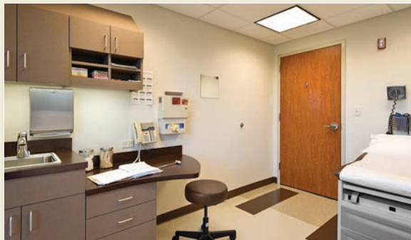
Aside from the lowered counter height, the most noticeable universal design feature shown is the wider door with a levered handle, making it easy to open for people of limited or full capabilities. (Photo: Dennis Jourdan)
