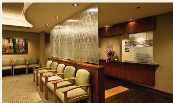
This waiting area features a lower counter height so anyone can check in easily regardless of abilities; wide traffic areas that allow for easy navigation by foot or wheelchair; and the chairs have arms well forward and space underneath to make them easier to access. (Photo: Loewenstein)
