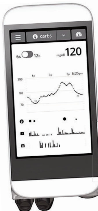
The iLet houses two independent pumping systems, one for insulin and one for glucagon. These pumps are automatically commanded by insulin and glucagon dosing algorithms every 5 minutes.
